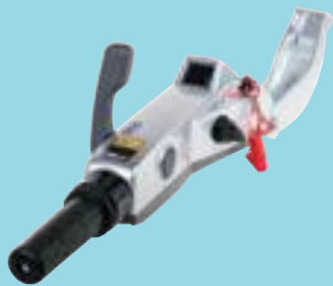
Multi-function Tiller Handle (BF40D & BF50D)
